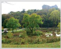
Philadelphia constructed the one-acre Saylor Grove stormwater wetland in a park area to collect and treat 70 million gallons of urban stormwater generated in the storm sewershed each year.
