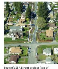
photo) uses numerous LID practices including rain gardens, vegetated swales and a narrow, winding street. A typical Seattle street (bottom of photo), by comparison, has a broad, wide street and flat yards with few natural depressions to capture and store stormwater runoff.
