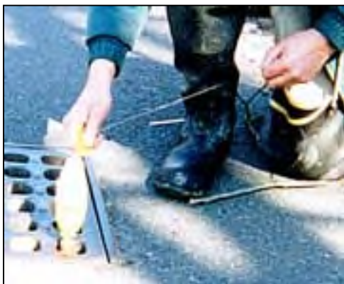
Figure 60: Optical Brightener Placement in the Storm Drain
