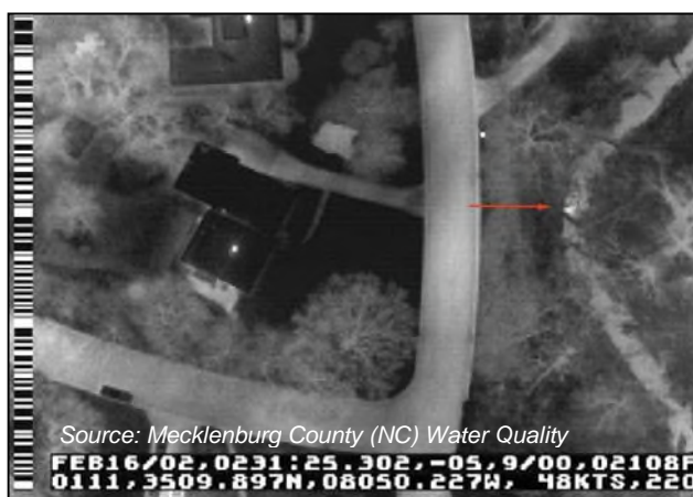
Figure 74: Aerial Thermography Showing Sewage Leak
